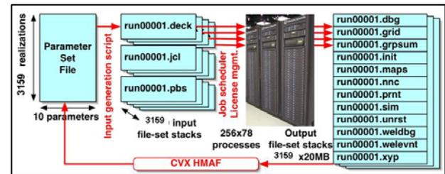
**Fig. 2 the 256 CPU Linux cluster at USC used for History Match using High Performance Computing (HPC) – from ref. 40.**
