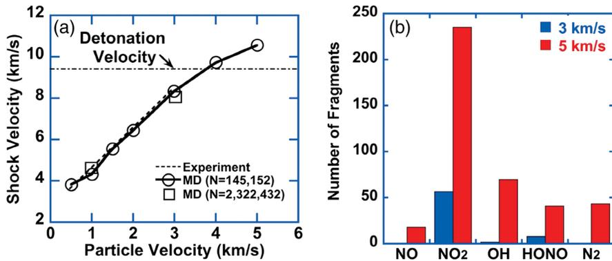
FIG. 2 (color). (a) Molecular dynamics (circles with solid lines to guide the eyes for  $N = 145, 152$  atoms and squares for  $N = 2, 322, 432$  atoms) and experimental (dashed) Hugoniot curves (particle velocity  $V_p$  vs shock velocity  $V_s$ ) for the RDX crystal. (b) Number of molecular fragments (for  $N = 145, 152$  atoms) produced during 1 ps after shock loading at  $V_p = 3$  km/s (blue) and 5 km/s (red).
