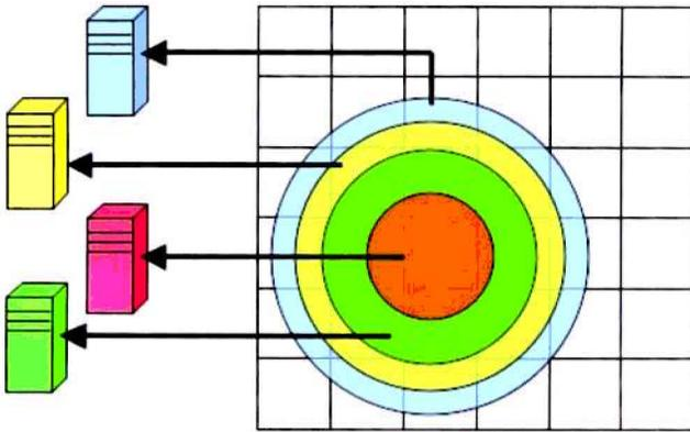
**Figure 3.** The parallel implementation of the octree-based view frustum culling. The concentric shells, each of equal volume, is distributed over a PC cluster to perform a coarse extraction of octree regions.
