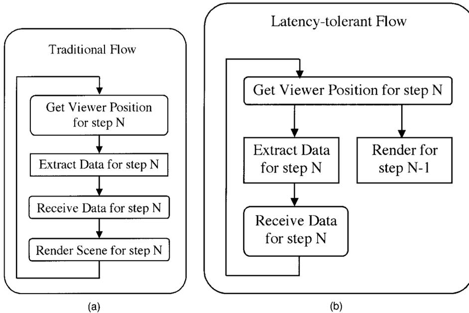
**Figure 6.** Dataflow overlapping communication and computation (right) is contrasted with traditional dataflow (left).
