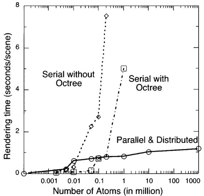
**Figure 7.** Rendering time per scene as a function of the number of atoms for the parallel and distributed Atomsviewer is compared with those for the serial Atomsviewer with and without the octree enhancement.
