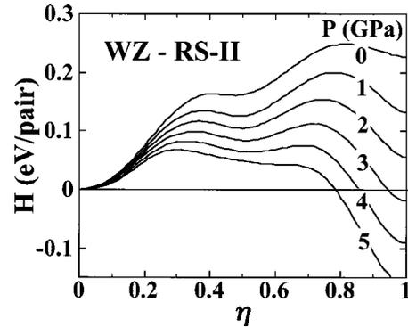
FIG. 4. Enthalpy as a function of pressure along the transition path from WZ ( $\eta=0$ ) to RS-II ( $\eta=1$ ) through HS ( $\eta=0.5$ ).
