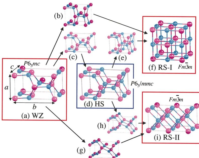
FIG. 2. (Color) Summary of the structural transformation from the wurtzite to the rocksalt structures in CdSe observed in our MD simulations. Each figure shows atomic configuration in the orthorhombic unit cell of CdSe. The magenta and blue spheres show the positions of Cd and Se atoms, respectively.
