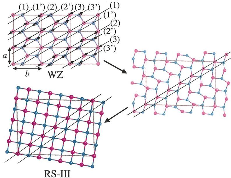
FIG. 7. (Color) The mechanism of the structural transformation from WZ to RS-III. The magenta and blue spheres show the positions of Cd and Se atoms, respectively. The small arrows in the WZ structure show the directions to which the internal atomic coordinates are shifted.
