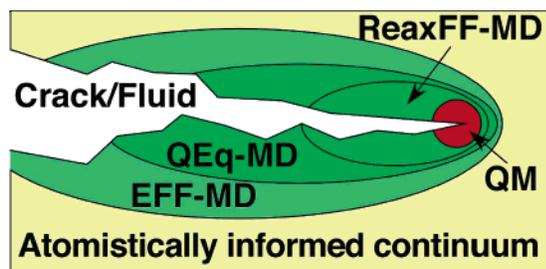
**Figure 1.** Hierarchical molecular dynamics simulation approach to fracture. Quantum mechanical and ReaxFF-MD computations are performed to study environmental effects on the crack tip. ReaxFF-MD is matched to QEq-MD and to EFF-MD in the process zone. Atomistically informed continuum models are compared with engineering fracture data.
