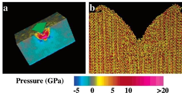
**Figure 6.** (a) Half-slice view of pressure in a silicon nitride sample during nanoindentation. (b) Atomic view showing amorphization under the indenter and material pileup at the edges of the indenter. Red and yellow are silicon and nitrogen atoms, respectively. These figures demonstrate the relationship between residual stresses and atomistic-level amorphization phenomena.
