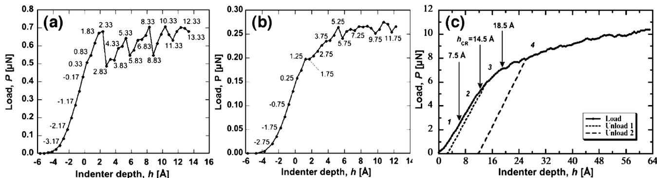
**Figure 7.** Load–displacement curve during indentation of (a) crystalline, (b) amorphous, and (c) nanocrystalline silicon carbide.
