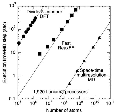
**Figure 3.** Benchmark tests of reactive and nonreactive MD simulations on 1920 Itanium2 processors of Columbia. The figure shows the total execution time per MD step as a function of the number of atoms for three linear-scaling algorithms: quantum-mechanical MD based on the divide-and-conquer density functional theory (circles); fast reactive force-field MD (squares); and space–time multiresolution MD (triangles). Lines show ideal  $O(N)$  scaling.
