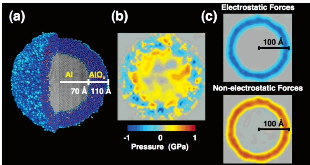
**Figure 5.** (a) Snapshot of the Al nanocluster after 0.5 ns of canonical MD simulation time. (A quarter of the system is cut out to show the aluminum/aluminum oxide interface.) The larger spheres correspond to oxygen, and smaller spheres to aluminum; color represents the charge on an atom. (b) Local pressure in the nanocluster after 100 ps of simulation time. (c) Electrostatic and nonelectrostatic contributions to the local pressure in Figure 5b.
