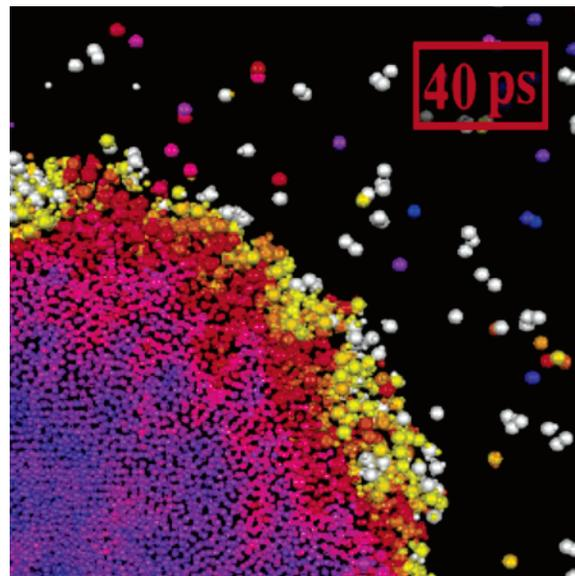
**Figure 4.** Temperature of atoms during the microcanonical MD simulation of an Al nanoparticle in an oxygen environment. The larger spheres correspond to oxygen, and smaller spheres to aluminum; color represents the temperature
