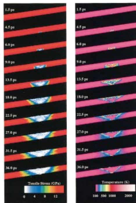
FIG. 4. (Color) (a) Time progression of local tensile stress of the 1204-chain nanowire; (b) time progression of local kinetic temperature of the 1204 chain nanowire.
